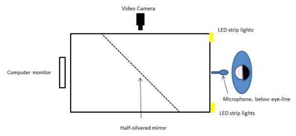
Figure 3 half-silvered mirror video capture setup
